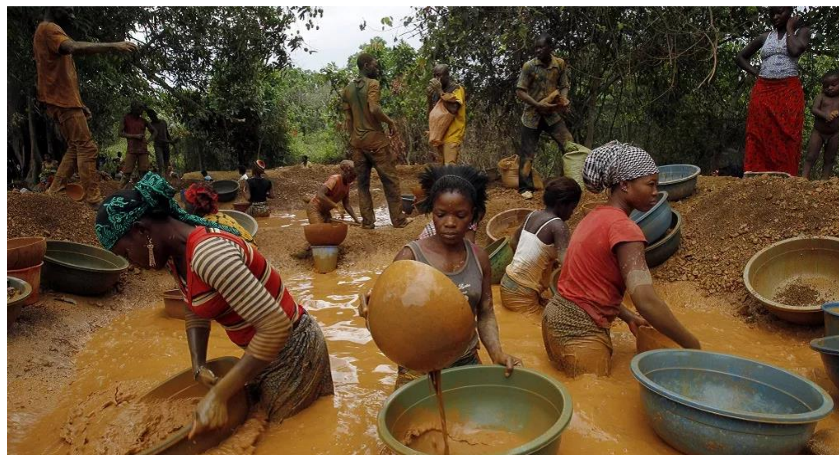
Figure 1. Illegal small-scale mining activity in a typical mining community in Ghana. Various techniques are employed in the mining activities including the use of mercury in the extraction of the gold. This type does not involve the use of technology as the miners are not able to employ such heavy-duty equipment for their mining activities. Source: https://static.euronews.com/articles/361915/1024x538_361915.jpg?1490806772
