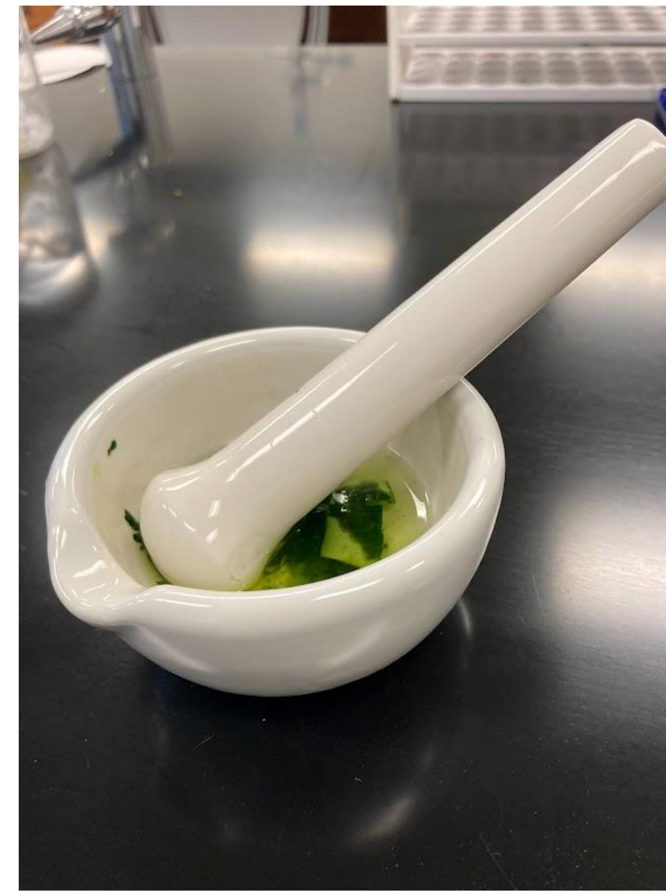
Figure 1. Preparation of peroxidase Samples of vegetable skin and sample buffer crushed with mortar and pestle to form final sample that will be used for purification.
