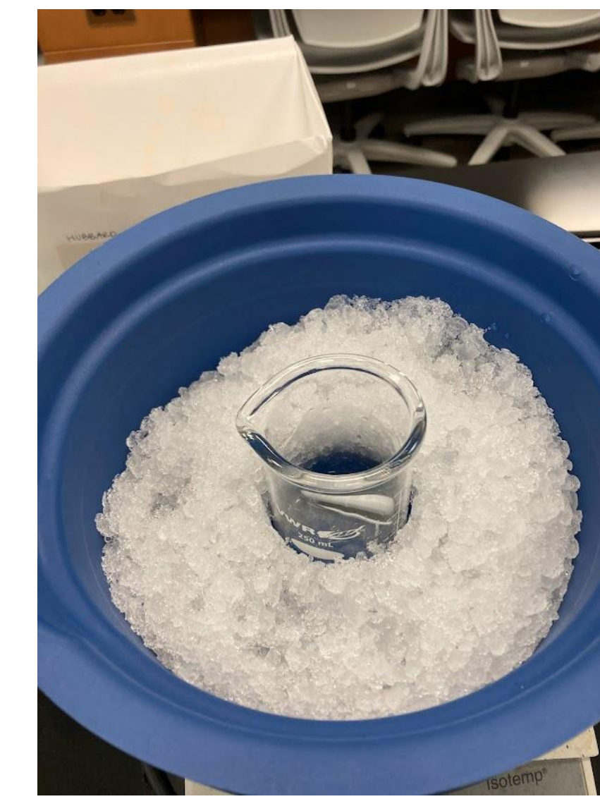
Figure 2. Purification process Purification was done by means of adding ammonium sulfate to a beaker of the peroxidase sample in an ice bath. This was followed by use of giant centrifuge to remove any precipitate or plant residue left over.
