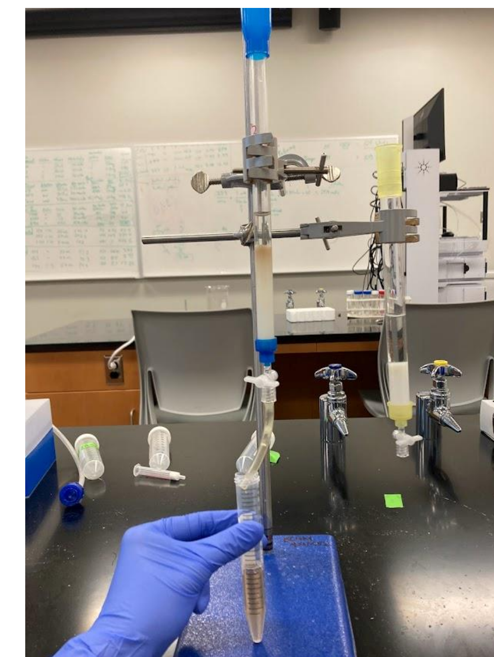
Figure 4. Column collection fractions Different fractions were collected as purified samples of peroxidase with ammonium sulfate were run through a column, collecting the sample from the solution. Then water was run to collect the sample and was eluted in different fractions which held enzymatic activity.
